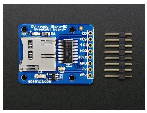
If you have a project with any audio, video, graphics, data logging, etc in it, you'll find that having a removable storage option is essential. Most microcontrollers have extremely limited built-in storage. For example, even the Arduino Mega chip (the Atmega2560) has a mere 4Kbytes of EEPROM storage. There's more flash (256K) but you can't write to it as easily and you have to be careful if you want to store information in flash that you don't overwrite the program itself!
