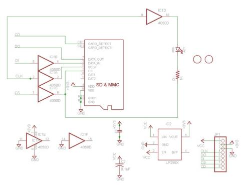
For the level shifter we use the CD74HC4050 (https://adafru.it/Boj) which has a typical propagation delay of ~10ns
