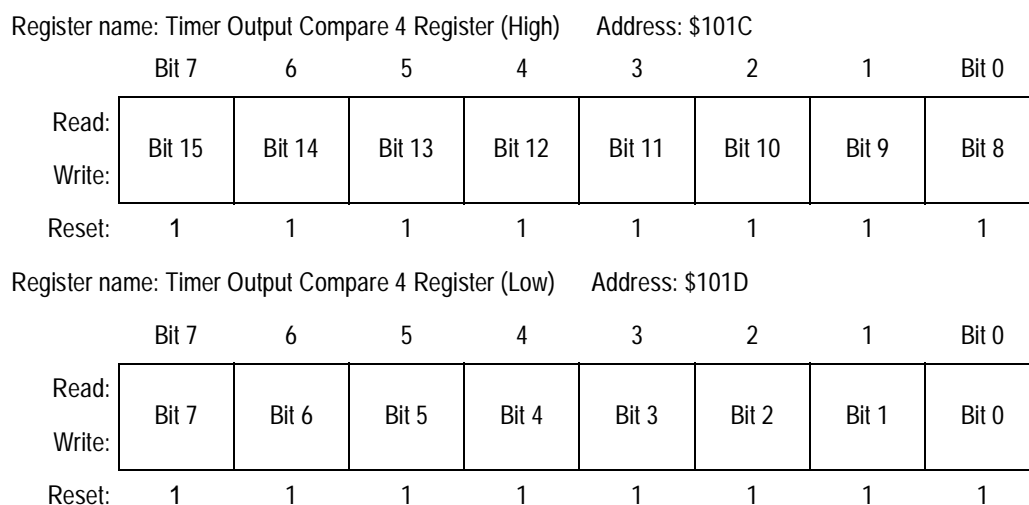
Figure 9-11. Timer Output Compare 4 Register Pair (TOC4)
