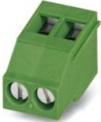
PCB terminal block, Nominal current: 24 A, Nom. voltage: 400 V, Pitch: 5 mm, Number of positions: 2, Connection method: Screw connection with tension sleeve, Mounting: Wave soldering, Conductor/PCB connection direction: 90 °, Color: green, The article can be aligned to create different nos. of positions!
