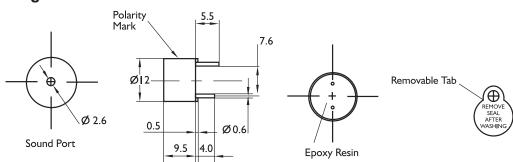
Dimensions : Millimetres Tolerance : ±0.5mm
